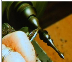
Making a fine finial for an ornament and turning the body. Edges at 45°.
