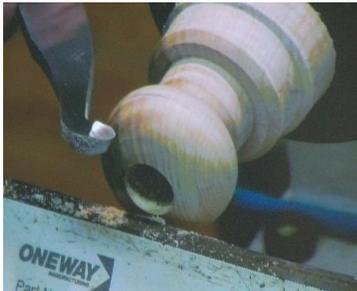
Using a hooked hollowing tool to hollow the inside of the ornament.
