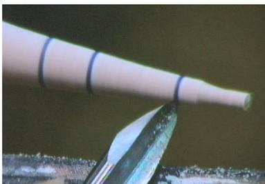
Mark the finial where the features should be. Notice the swept back grind on the spindle gouge.
