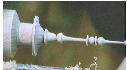
The completed finial, ready to be parted off and fitted to the ornament body. Note the cap of the finial was measured to fit the body.
