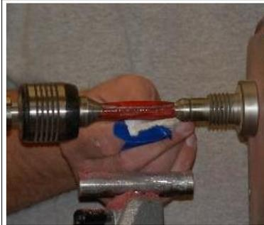
Applying the specially formulated CA glue. It dries slower and is more flexible than standard CA.
