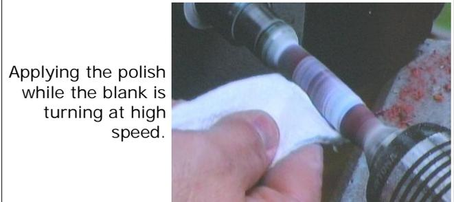
Applying the polish while the blank is turning at high speed.
