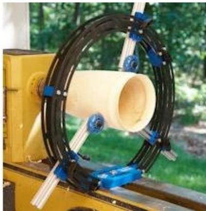
The other section covers from 10:00 around to 5:00 on the top and front and completes the circle. The top front portion is bolted at the top and hinged at the lower front. Remove a bolt at the top and it swings forward and is then easily removed.
