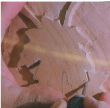
Laying the shape of two overlapping leaves out on a disc. Removing some wood from the surface around the outside of the first leaf, and beginning to outline the 2nd leaf.
