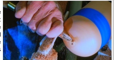
Finishing off the top with it taped to the base (no tail stock possible for this
