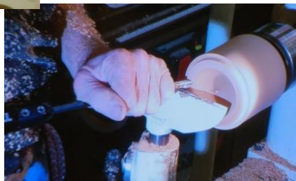
Working on the base and getting the lip for the top correct.
