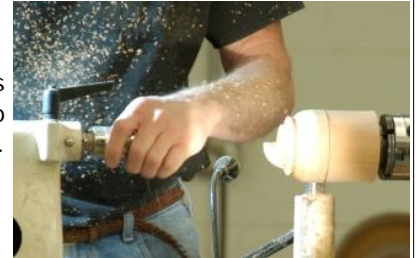
Shaping the top as it is jammed on to the base.
