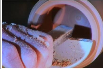
Using a round nose scraper to clean up the bottom of the inside of the base.
